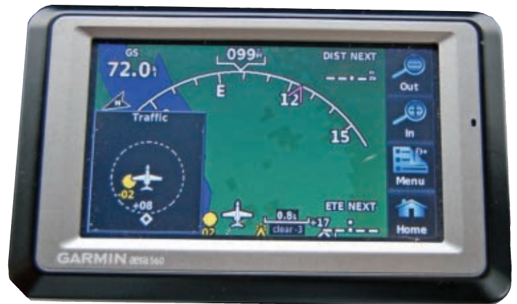
Regardless of which Aera GPS page is displayed, when an aircraft gets close, a Traffic Warning Window appears in the lower left. Note it shows a second aircraft at 6 o'clock that doesn't appear on the main map, since the airplane symbol is placed near the bottom of the display.
