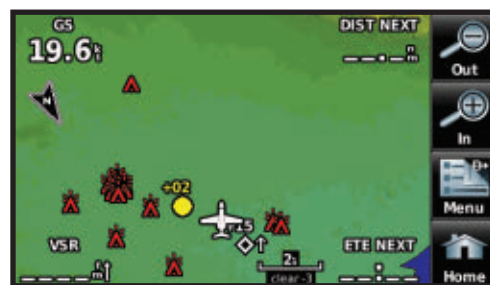
The XRX prioritizes aircraft primarily by their relative altitude. In this case, the 10 o'clock traffic triggered a traffic alert since it's 200 feet higher. The 4 o'clock traffic is closer but 1,500 feet higher and climbing.
