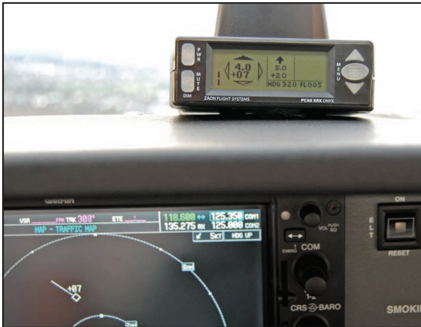
The G1000 shows an aircraft 3.2 miles away and 700 feet higher. The XRX shows the same aircraft 4 miles away and a second aircraft 2,000 feet higher and 5 miles away. That second aircraft was probably farther out than the 6-mile range displayed on the G1000.
