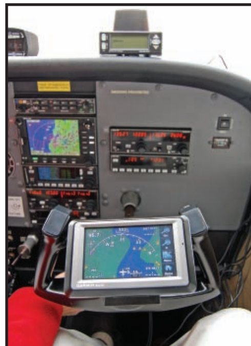
This otherwise well-equipped Cessna 172 lacked a traffic system. The Zacon XRX needs to be mounted level on the glare shield and at least 6 inches from the compass and other metal objects.
